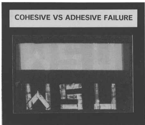
FIGURE 11 Cohesive-adhesive failure. A sandwich of Magic Tape was separated while it was held in close contact with the Type 107C Film by Double Stick Tape. The letters WSU were regions where the magic Tape peeled from its backing, surrounded by adhesive-from-adhesive peeling.
