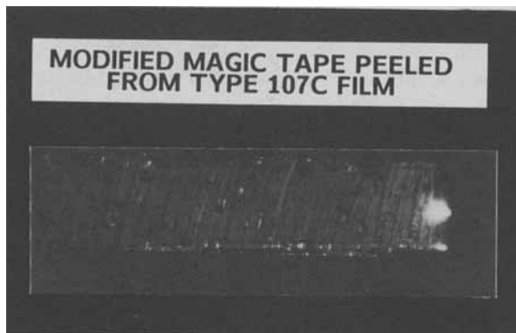
FIGURE 4 Magic Tape stiffened by two layers of electrical tape then peeled from Type 107C Film.
