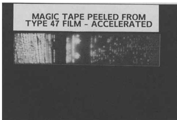
FIGURE 8 An example of complex discharge activity during peeling. Magic Tape peeled from Type 47 Film at an increasing speed.
