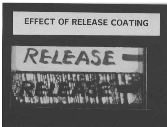
FIGURE 13 A release coating of ink from a felt tip pen was applied to the adhesive surface before the joint was made (Staedtler Lumocolor pen was used). The ink decreased the adhesion by a factor of five and greatly suppressed the light emission. The reconstructed sample is shown on the top.
